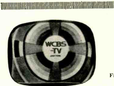
Fig. 3—Picture is improperly centered.
