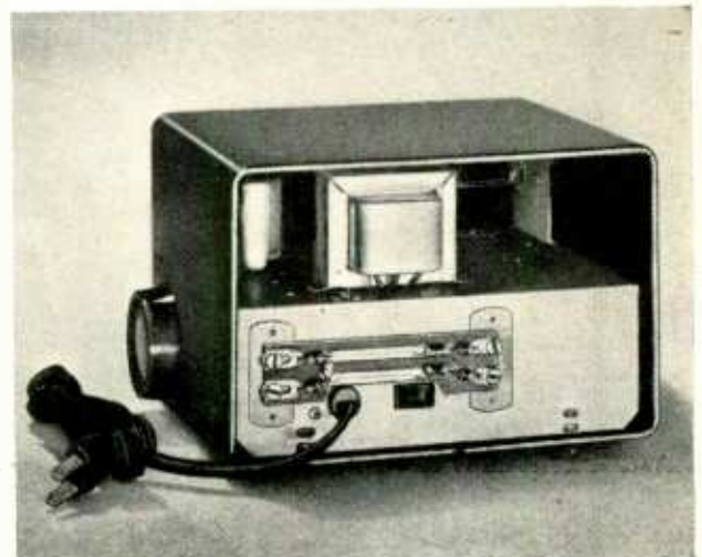
Rear view of the booster, showing the v.h.f. bypass filter in place.
